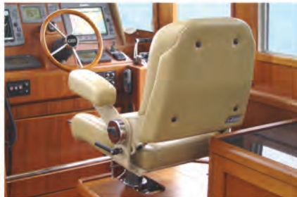
Cabinet space with a view! Top: Two 500N Slimlines with deck penetrating telescoping pedestals aboard an MJM 34Z. Right: The helm of the Grand Banks 55 Eastbay SX features a deck penetrating pedestal which provides an adjustable seat height for better visibility.
