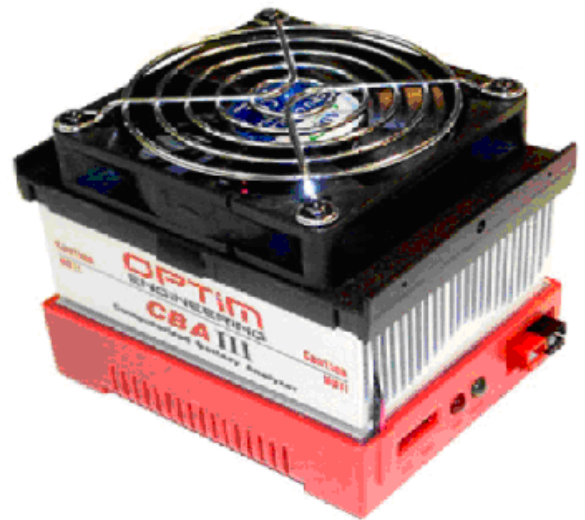
CBA III Computerized Battery Analyzer for any type or size of battery, up to 55 volts, 150 watts, or 40 amps. Runs on your computer through a USB connection. About $150
