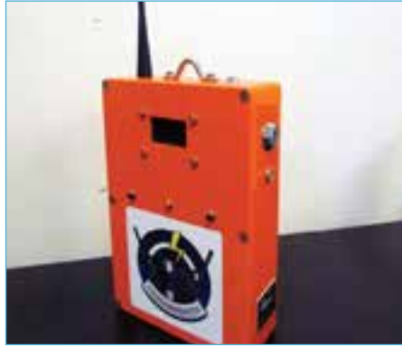
RADIO REPEATER The Radio Repeater mode retransmits master controller radio signals for starting & ending games - place the repeater on high ground with clear lines of sight. (GG REPEATER).
