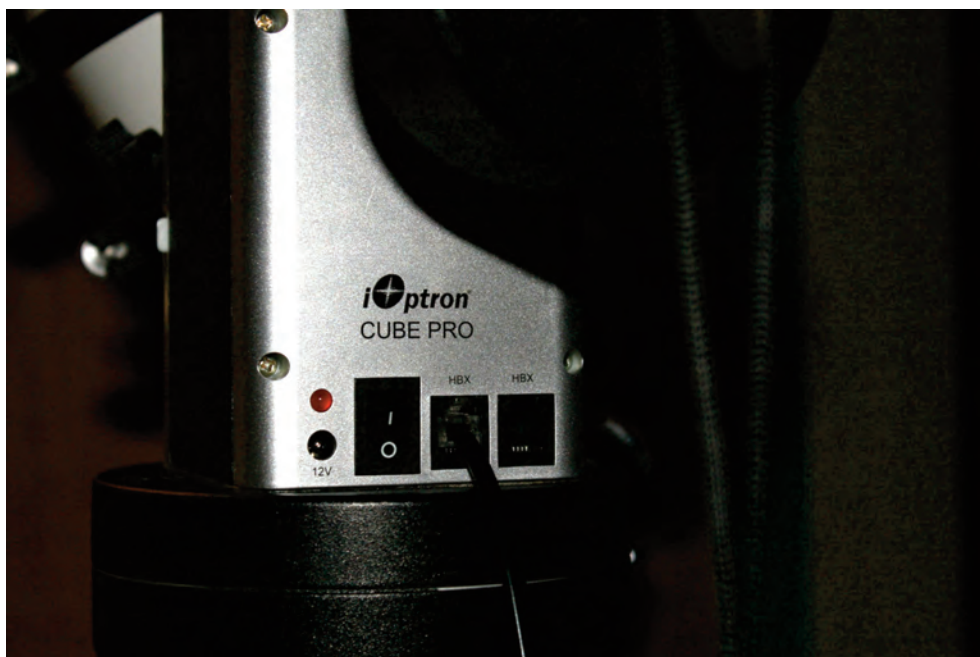
Image 7 - This side of the Cube has the on/off switched, a red lamp that is illuminated when the power is on, a 12-volt jack for connecting a power cable (if not using batteries in the internal battery compartment), and two HBX outlets.
