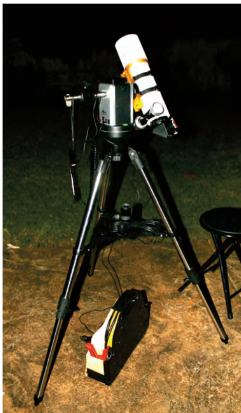
Image 3 - The completely assembled iOptron Cube mount with a William Optics Star 71 apochromatic refractor.
