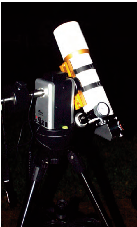
Image 4 - The small black box on the top of the Cube housed the GPS receiver.
