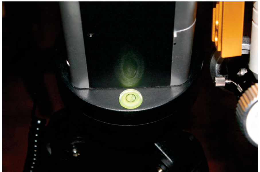
Image 5 - A close up of the bubble level built into the top of the Cube's base.
