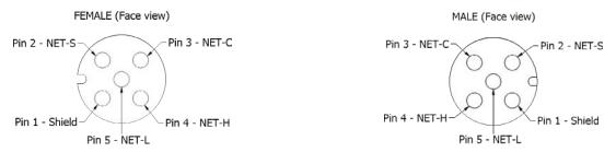
An Actisense Panel Mounted Wire (PMW) connector is a great tool for plugging in to a spare T-piece to quickly identify the correct pins via the wiring colours. It is recommended that each wire from the PMW is terminated inside a terminal block prior to plugging it in to the network as voltage may be present across the NET-S and NET-C pins.
