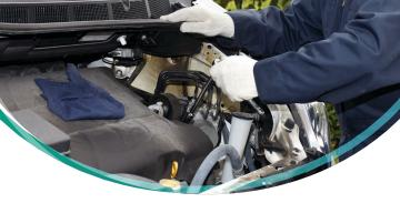
**Battery** – Powers the starter motor, acts as a voltage stabilizer for the electrical system and makes up any shortfall when the alternator cannot meet the vehicle's electrical demands. Inspect the battery cable connections at every oil change and clean as needed. Always wear eye protection and gloves when servicing a battery.
