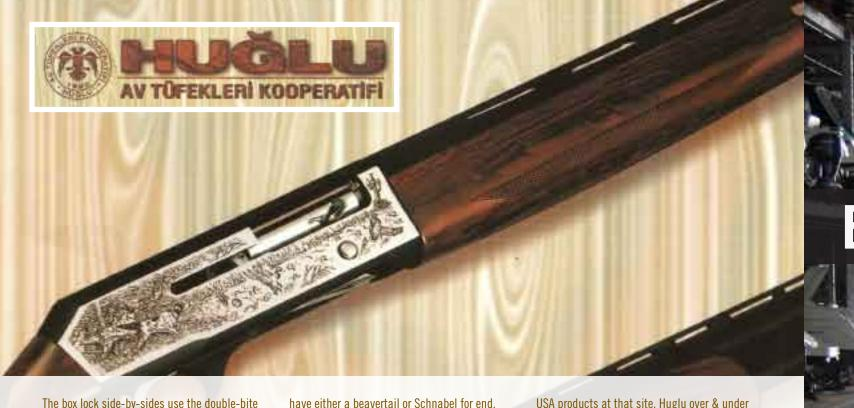
chopper-lump system and a cross bolt through the barrel extension. It is one strong-looking setup. I'd say you would have a hard time shooting a Huglu side-by-side loose. They are available in 12, 16, 20 and 28 gauges. Receivers are scaled to the gauge.
