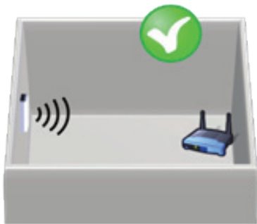
Antenna in vertical position and pointing to the Wi-Fi Access Point or Router.
