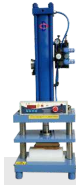
Hydraulic Cylinder Operated Press Machine for Specimen Die Punching Application
