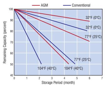
This chart illustrates how temperature and type of battery effects battery capacity. Colder storage temperatures are best for long-term storage. For example, an AGM battery stored at  $32^{\circ}$ F holds 90% of its capacity for about 6 months. The same battery stored at  $104^{\circ}$ F loses 50% of its capacity in 4 months. These temperatures can be reached if the battery is stored in garage or shed in hot weather.
