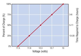
The approximate charging times are shown using a constant current charger (smart charger) at the amps specified on the battery.
