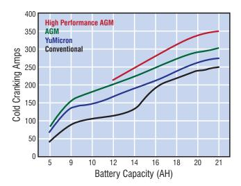
Battery design as well as materials used in construction give each type of Yuasa battery different performance ratings. This chart shows the relationship between battery capacity in amp hours and cold cranking amps.
