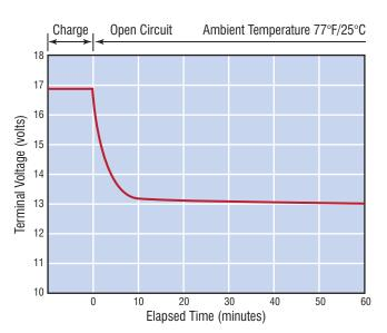
During the initial charging period, battery voltage may reach over 16-volts. Open circuit voltage should be checked after the battery is allowed to stand between 1 and 2 hours.
