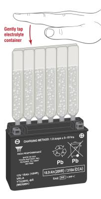
5. Remove the empty electrolyte container from the battery. Fully insert the strip of sealing caps (previously removed from the electrolyte container) into the battery filling ports. Make sure the strip of caps is fully inserted and flush with the top of the battery. Insert the caps by hand, do not use
