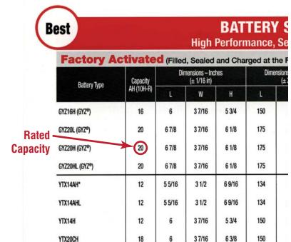
The Yuasa Battery Specifications & Applications guide lists information including: Battery Type, Dimensions and Capacity in Amp Hours (AH).
