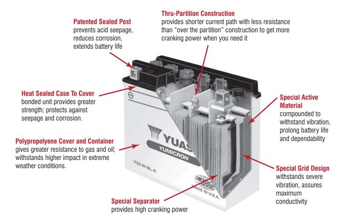
Yuasa batteries are also available as a dry battery with an acid pack. The part numbers for these batteries end with "-BS" to signify "bottle supplied" (i.e. YTX14-BS, YTX20HL-BS). Because the battery is shipped dry, it has an indefinite shelf life before it is activated as long as the foil covering the cells remains intact, undamaged and air-tight.
