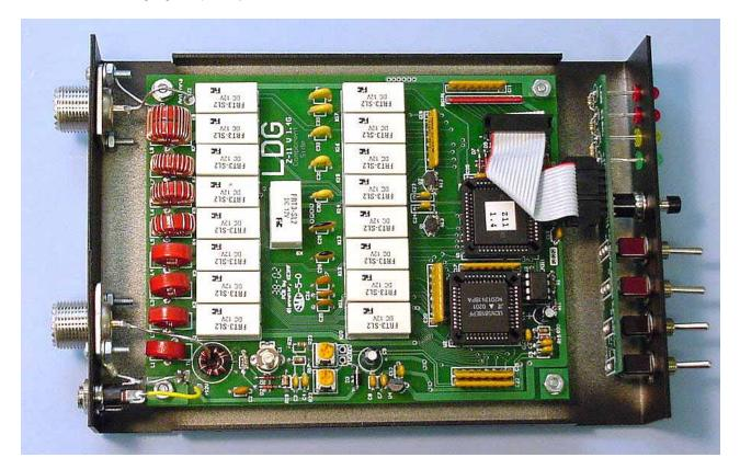
**One Touch Tune (OTT) Operation**: The Z11 can also be interfaced to directly control an FT-817. The One Touch Tune interface from W4RT Electronics (<u>www.w4rt.com</u>) can be purchased separately. With the OTT installed, the user simply presses the tune button the Z11 and the OTT sends a command to the 817 to transmit a carrier while the tuner is tuning. While not required for operation with the FT-817, the OTT makes changing bands and re-tuning a snap.
