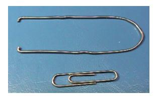
The extraction tool fits into opposite corners of the 68HC11socket; the bent ends will lift the chip from beneath. Touch a ground point to avoid static discharge damage, and remove the case top. Insert the tool and pull gently and evenly on both sides to extract the chip. Press the upgrade chip into the socket, observing the small diagonal corner key. Replace the case top; your upgraded Z11 is ready for service.
