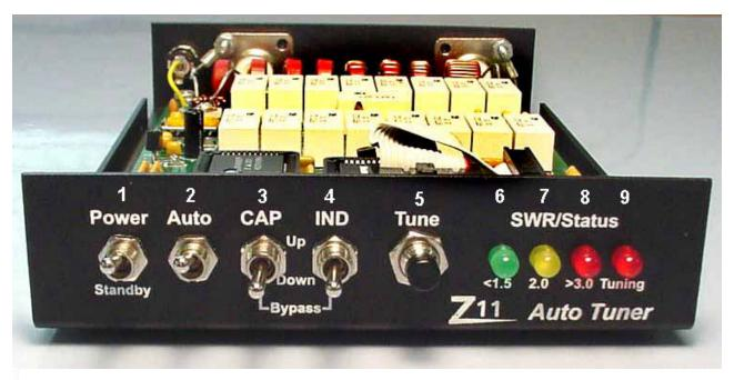
**Power/Standby**: The Power/Standby switch (1) turns the unit on and off. In Power position (up), the Z11 is on, and in Standby position (down), off with zero current draw. Remember, after tuning you can set this switch to Standby, eliminating current draw, and the latching relays will still retain their tuned setting.
