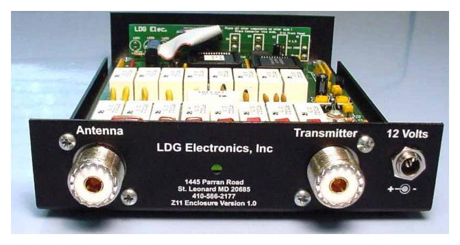
**Back Panel Connections**: The back panel has standard SO-239 jacks for connecting to the antenna and transmitter; use standard PL-259 plugs. A coaxial power jack (5.5 by 2.5 mm, center pin positive) provides DC power to the tuner. The power supply must provide between 11 and 20 volts DC at 200 milliamps for up to three seconds. If your transceiver or transmitter operates on 12 volts DC, the Z11 can be powered by the same source.
