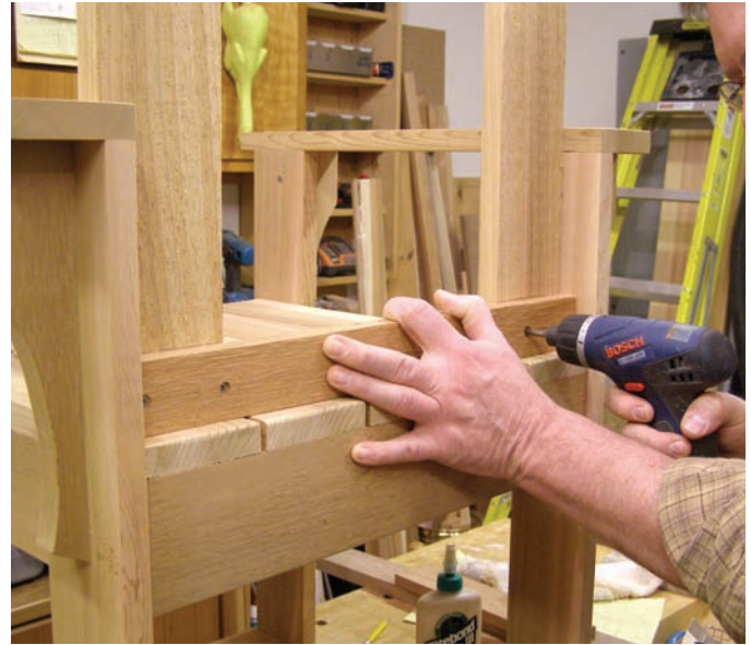
Although it isn't attached at this point, assembling the backrest inside the chair ensures a perfect, snug fit. Be sure the spacing of the backrest slats matches those in the seat.
