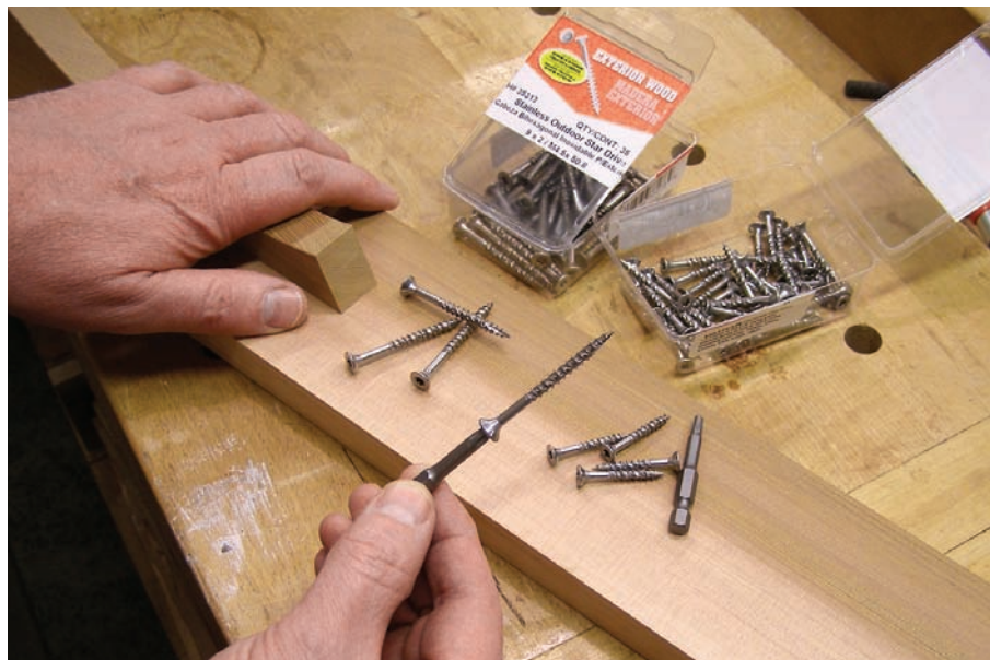
The stainless steel screws used for this project are self-drilling, and feature a star-drive head.
