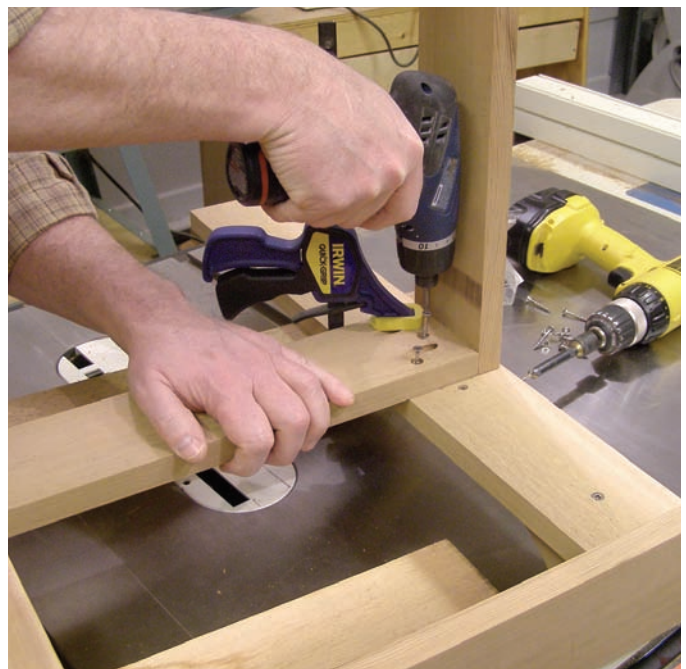
Attach the completed seat box to the leg sets with three countersunk 1\frac{1}{4} " screws. Scrap wood under the leg set keeps everything level.
