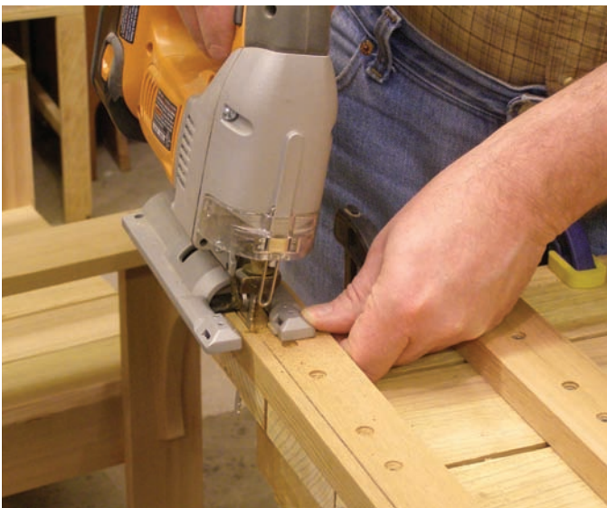
With the jigsaw set at 12°, cut the bevel into the bottom edge of the backrest.
