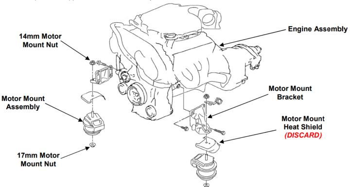
8. Once the motor has been reinstalled onto the engine's cross member, torque the lower nut to between <u>65-72ft-lbs</u>. Again, it is recommended that some form of thread locking compound be applied for additional security.
