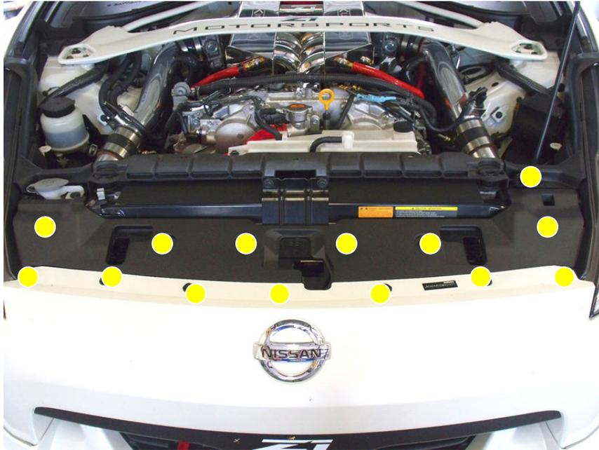
9. Remove the two 10mm Plastic Screws
