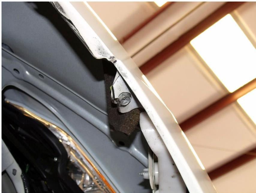
10. Gripping the sides of fascia (circled below) pull the fascia towards you. This part of the fascia snaps in place and will pop loose when a limited amount of force is applied. Once free, carefully remove the fascia from the chassis and set aside.
