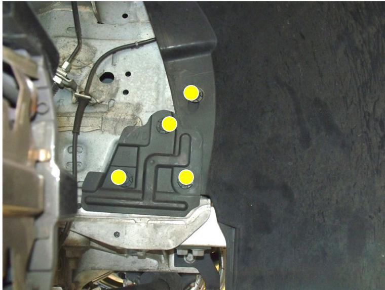
c. Be sure to remove these two plastic panel clips. The one shown in the image below on the Left will be exposed only after the lower engine shroud is removed. There is also a plastic panel clip (not shown) at the very top of the fender liner that will also need to be removed.
