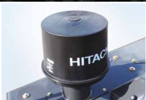
Less filter cleaning is required thanks to the optional pre-cleaner.
