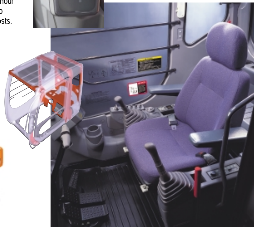
Cab design both guards the operator and contributes to efficient operation through its comfortable, ergonomic layout and its CRES design.
