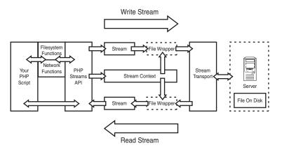
Figure 10.2 The PHP streams architecture.
