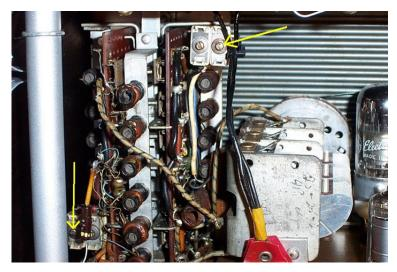
The 4-8Mc band also required the adjustment of trimmer capacitors, C33A, C36A & C37A (osc., det, & ant). Those trimmers sit right next to those for the 2-4MC band:
