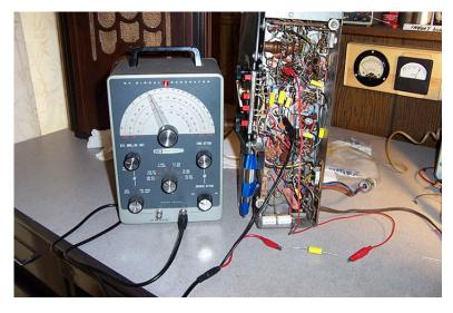
The sig. gen. was now feeding 455kc to the circuit, so it was time to peak out L5, L6, L7 and L8. They're the four slugs in the IF cans, two in each can. A 6-sided, non-metallic tool is needed to make the adjustments:
