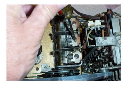
The final broadcast band adjustment is C32, located at the rear of the chassis. It's done with the signal generator and radio both tuned to 600kc.
