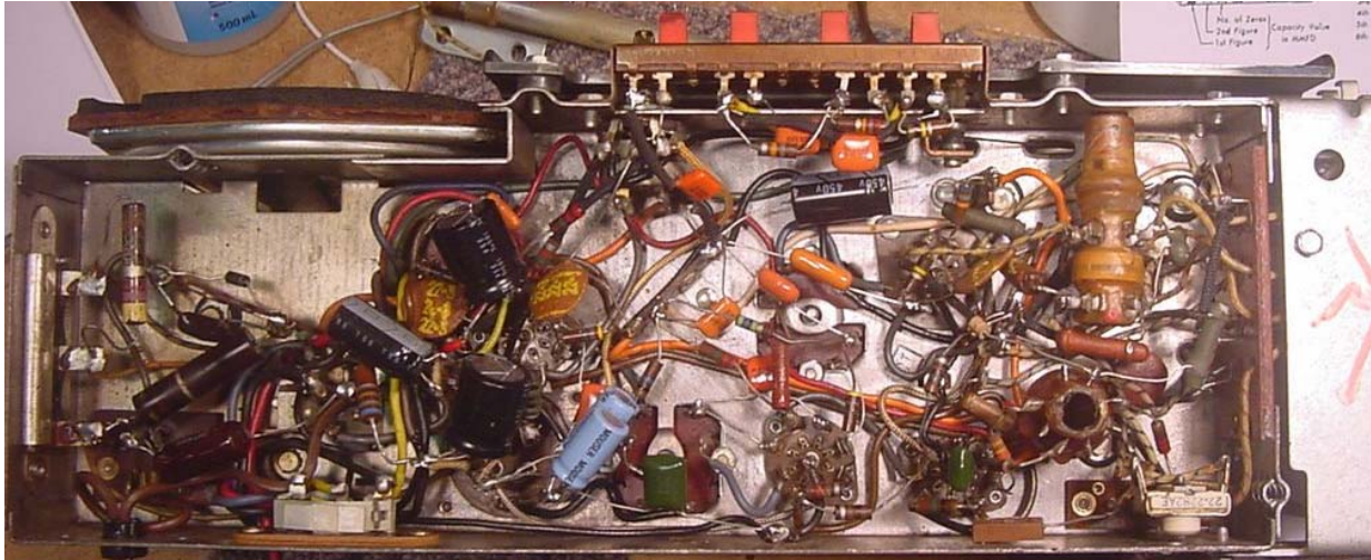
Above: Beneath the chassis after repairs, Note the ‘Bumble Bee’ and other paper capacitor types have been replaced by modern plastic film types (orange and green bodies). Below: Tuner section of the chassis – not quite as daunting as it looks – honest...
