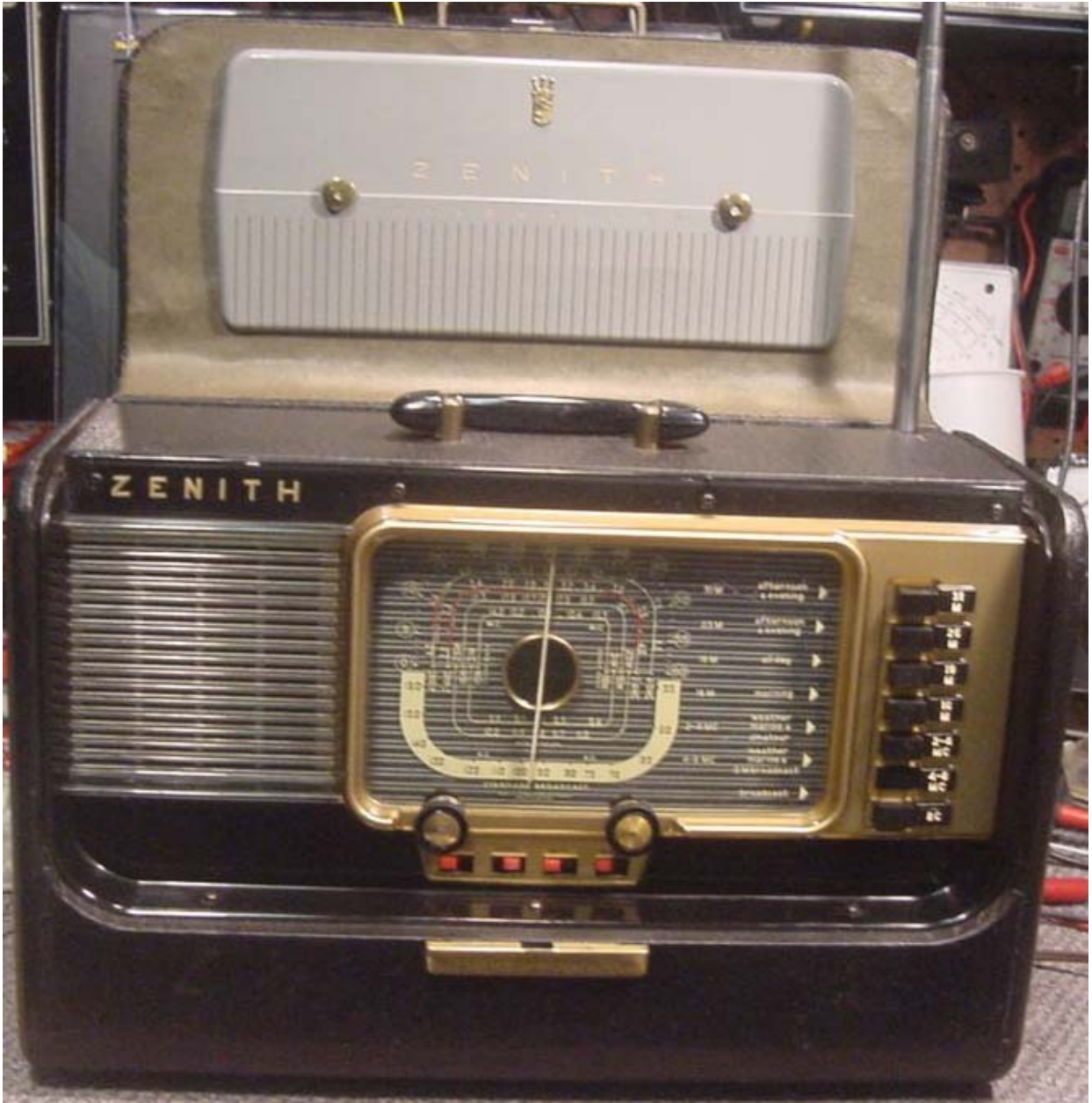
Restored Zenith Transoceanic H500 – pulling those distant stations in with ease and classic early-1950's style. Note the 'WaveMagnet' detachable loop antenna in the lid for Broadcast band reception and the extended 'WaveRod' (upper right) for shortwave reception
