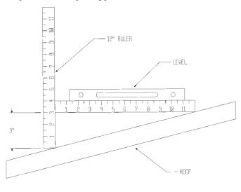
Continue adding lengths of vent until the proper height is achieved (See diagram above). Slide raincap into vent.
