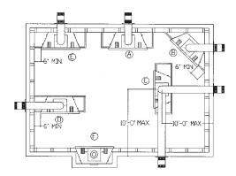
Island installation with a top vent is possible as long as the horizontal portion of the vent system does not exceed 10 feet (305cm). When you install your fireplace as in position 'B', 'D' or 'E', a minimum of 6 inches (153mm) clearance must be maintained from the perpendicular wall and the front of the appliance.
