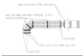
**NOTE:** It is critical to the proper and safe operation of this fireplace that on all connections the inner liner and the outer casing are both caulked with liberal amounts of sealant. Do not use any kind of tape or silicone other than that recommended in this manual. Mill Pac Sealant
