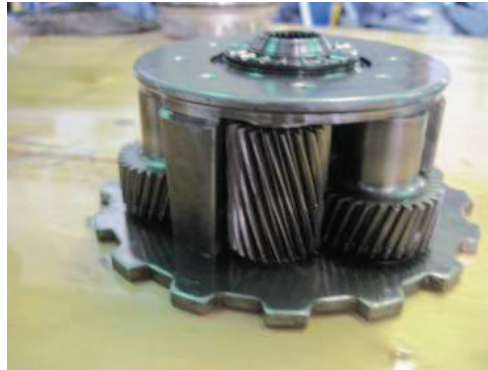
1 Planetary carrier holding: 2 sets of planets. Inner and outer planet
