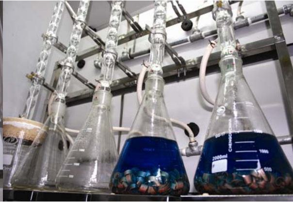
Intergranular Corrosion Test
