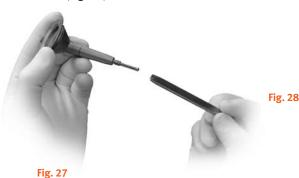
Attach the Humeral Stem Inserter/ Extractor to the trial assembly by opening the handle all the way, inserting the Inserter/Remover end into the proximal opening in the assembly, and closing the handle to lock the inserter in place (Fig. 28).
