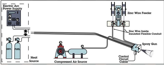
Figure 6: Zinc Spray Metallizing
