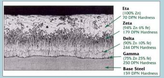
Figure 4: Photomicrograph of a Galvanized Coating
