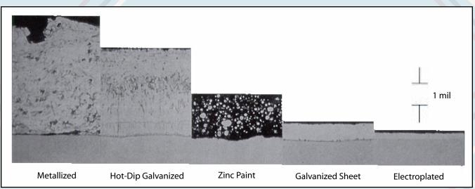
Figure 2: Microstructures of Various Zinc Coatings
