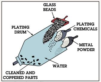
Figure 7: Mechanical Plating
