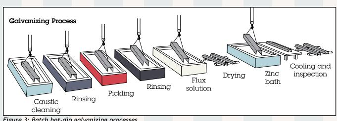
Figure 3: Batch hot-dip galvanizing processes
