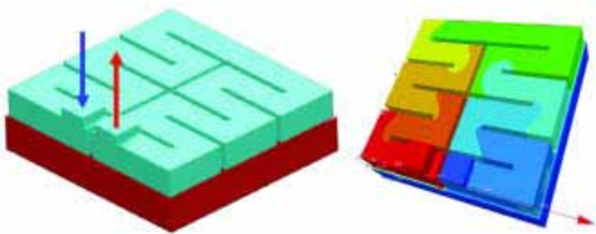
Figure 9. A unit meander cell, the liquid (blue) is placed on a piece of baseplate. To the right the pressure distribution is shown, found from a CFD simulation.
