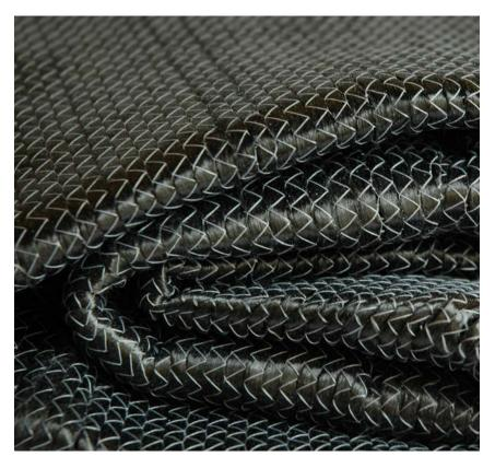
ZOLTEK PX35 Stitch-Bonded Unidirectional Carbon Fabrics are produced from our ZOLTEK PX35 50K Continuous Tow Carbon Fiber. Unique fiber spreading techniques are utilized to obtain a wide range of UD fabric weights for a varied set of composite part applications. Quick composite part build-up is cost effectively achieved with our diverse weight range of low-cost carbon fabric products.
