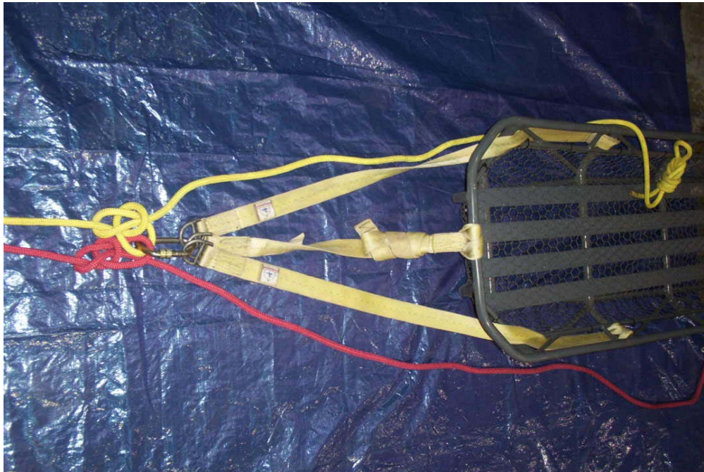
Two-rope system attachment to the head of a litter using a low angle evac harness for the yoke. (Bowlines shown tied loose for picture clarity).
