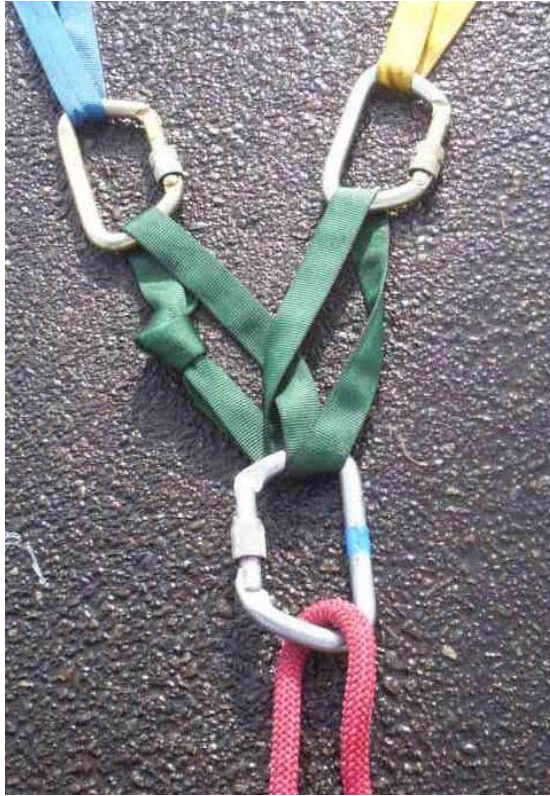
Two point load distributing using webbing.
