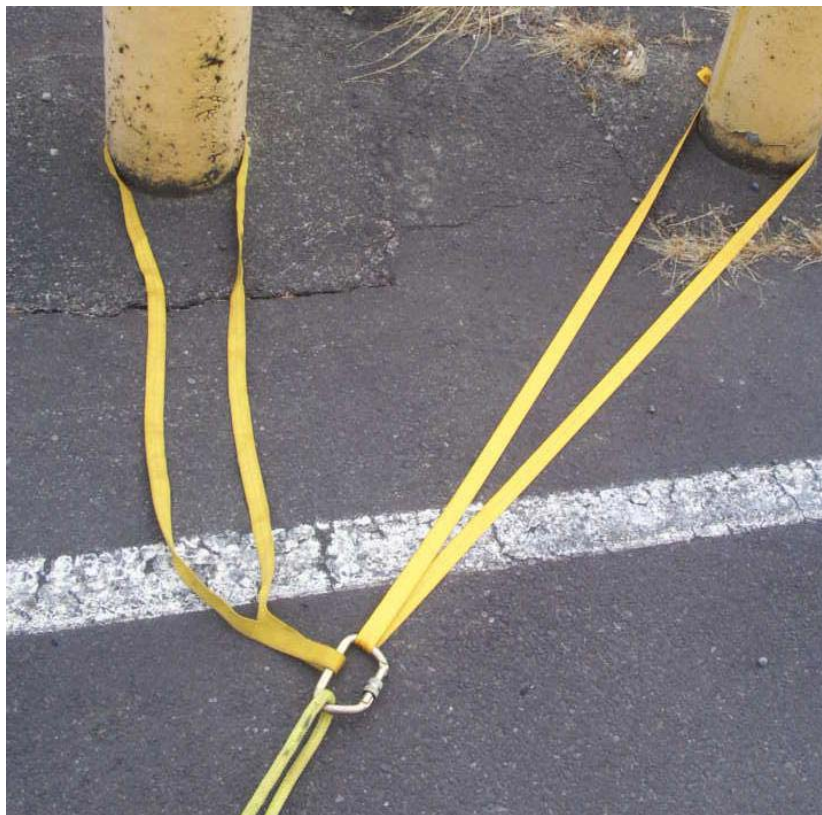
Load sharing anchor system with load shift
