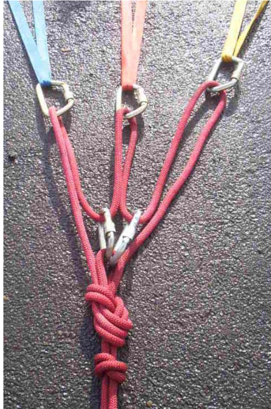
Three point load distributing using life safety rope configured with a Double Loop Figure-8.
