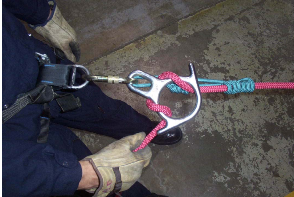
Descending with Figure 8 Plate and single Prusik.
