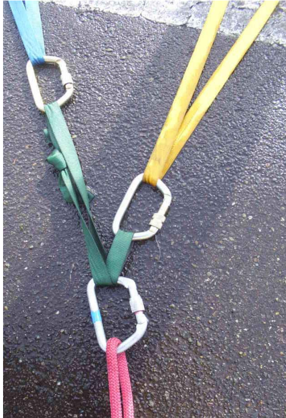
Two point load distributing with load shift.
