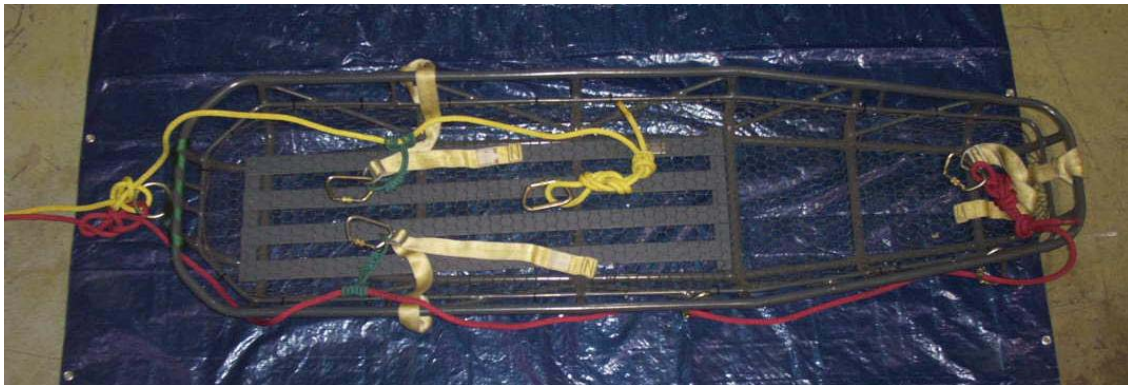
Litter Tender attachment for three rescuers on the litter using stretcher tender straps.
