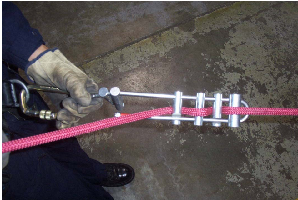
Descending with a Brake Bar rack
