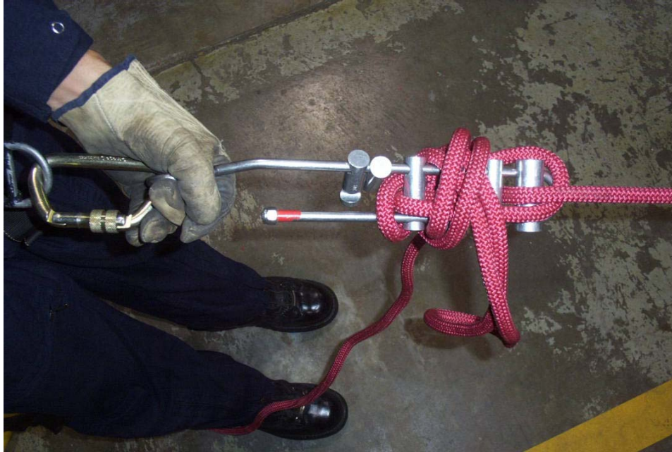
Brake Bar Rack locked off.
