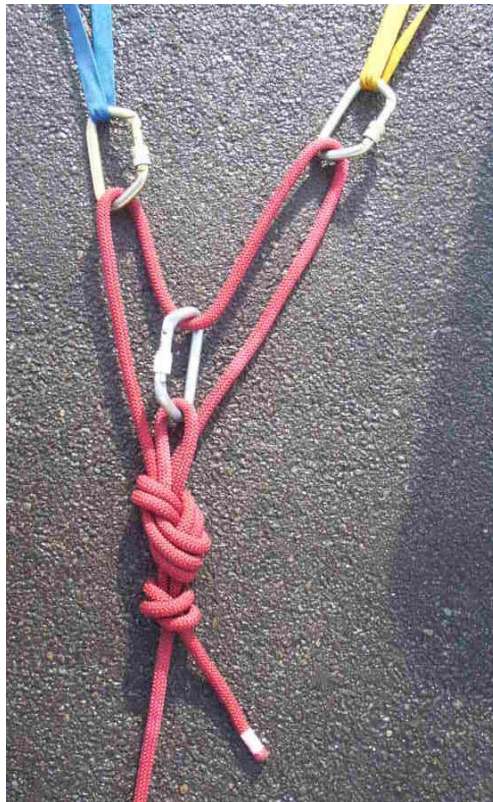
Two point load distributing using life safety rope configured with a Double Loop Figure-8.
