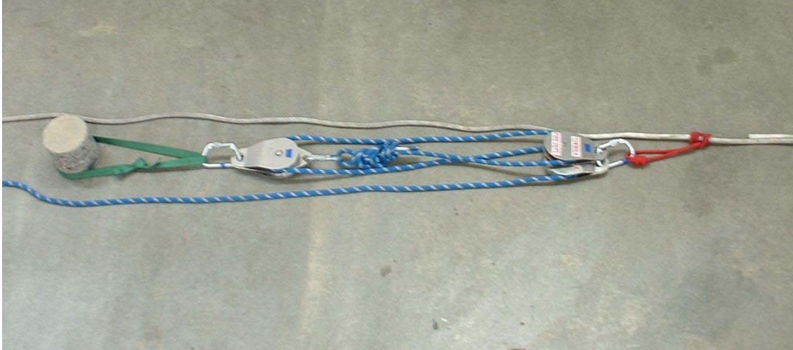
Pig Rig using a double sheave pulley and two separate pulleys to provide 4:1 MA Note: an additional double sheave pulley may replace the separate single pulleys
