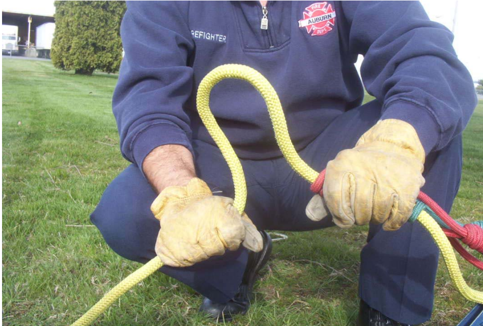
Operation of Tandem Prusiks on a lowering operation.
