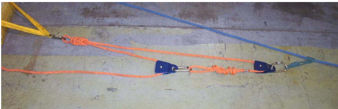
Pig Rig using two Prusik Minding Pulleys to provide 4:1 MA
