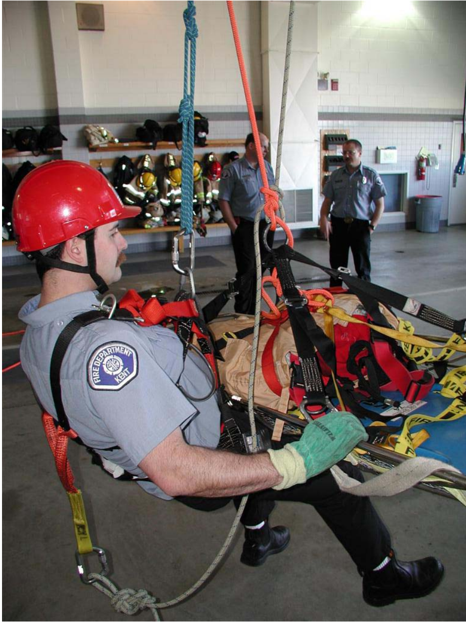
Tender attachment with a Purcell Prusik to the Main Line and tail from the Belay Lines Longtail Bowline.
