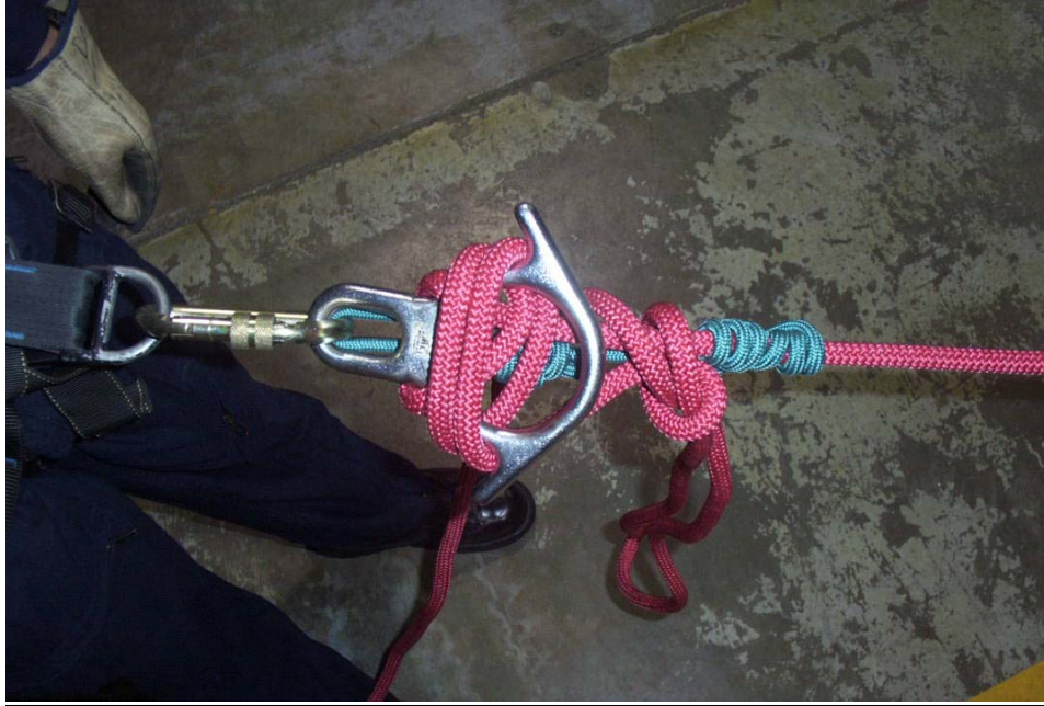
Figure 8 Plate locked off.
