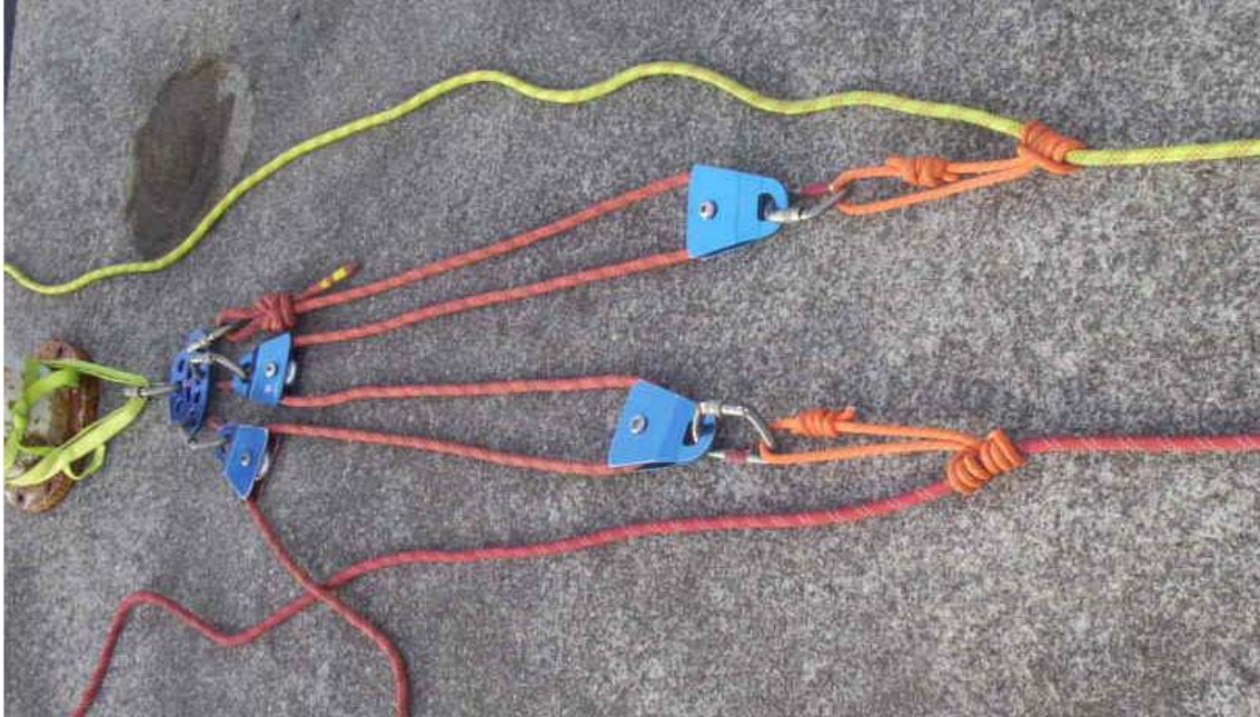
Tensioning system for Track Lines.
