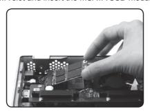
2. Gently press down on the mSATA SSD module and install the screw.
