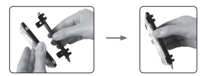
3. Insert the hard disk into the slot at a 45 degree angle and gently slide into the connector.
