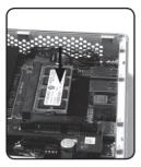
Note: This ZOTAC ZBOX accomodates two DDR3 SO-DIMM memory modules. You must install at least one module in one of the two slots.
