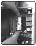
2. Remove the memory module from the slot at a 45-degree angle.
