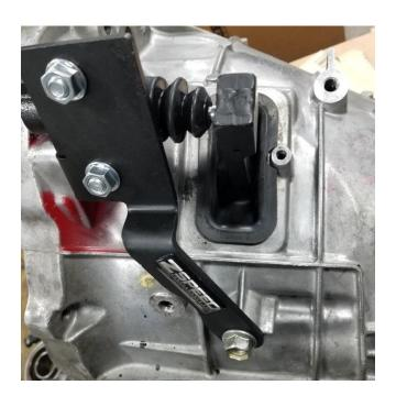
Install Stainless Clutch hose to OEM hard pipe and slave cylinder AND ROUTE AWAY FROM EXHAUST AND STEERING KNUCKLE. Remove the 1 or 2 metal harness brackets (depending on model) from starter harnesses and zip tie harness to slave bracket. You can route the harness between bracket and transmission.
