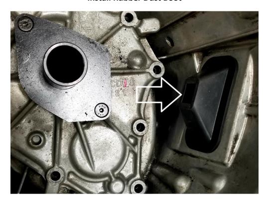
install CMAK Clutch Fork, Bearing and Bracket assembly with the QTY (5) 50mm long bolts, Slip fork and bearing assembly preassembled through dust boot.
