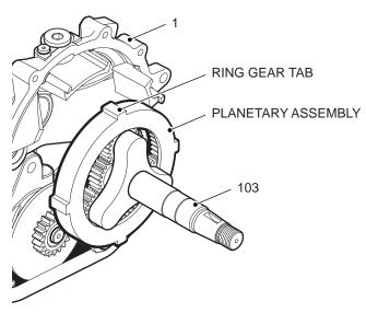
Figure 17, Planetary Gear Set
