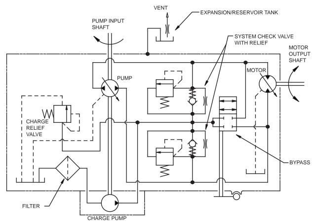
Figure 1, Hydraulic Schematic With Charge Pump
