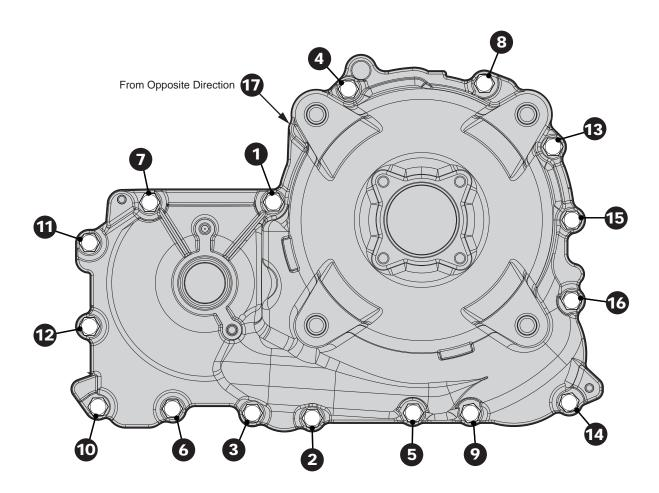
Figure 27, Screw tightening sequence
