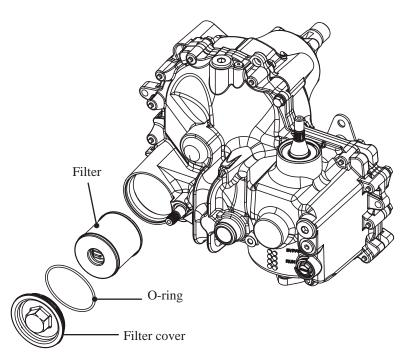
Figure 3a, Filter Components
