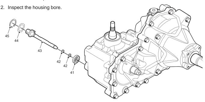
Figure 14, Bypass Actuator
