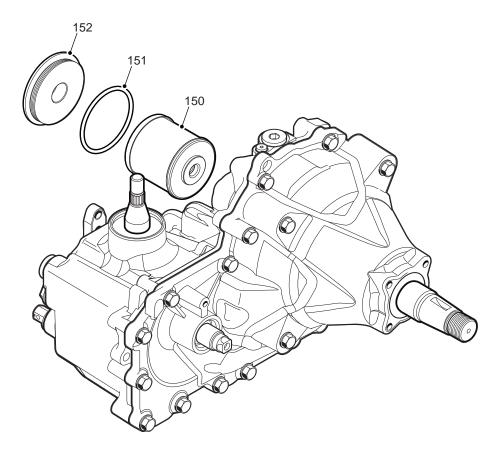
Figure 11, Filter and Filter Cover
