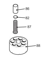
Figure 21, Pump Block Assembly
