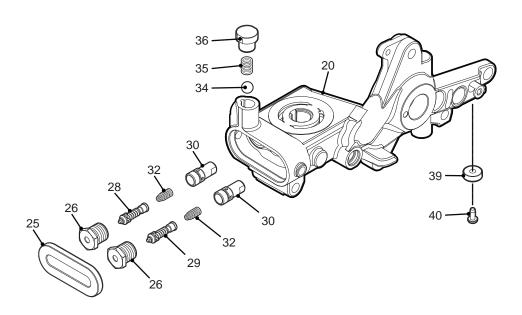
Figure 25, Charge Galley Assembly and Magnet
