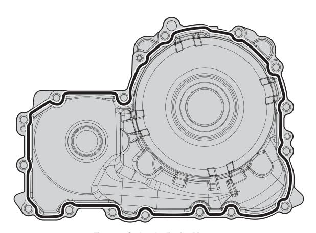
Figure 26, Sealant Application Diagram
