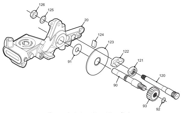
Figure 23, Brake Assembly and Motor Shaft
