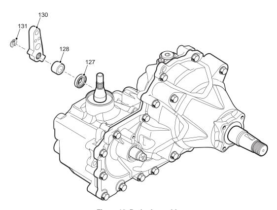
Figure 12, Brake Assembly
