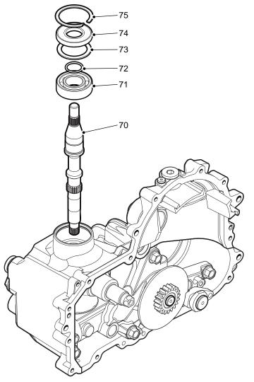
Figure 19, Input Shaft
