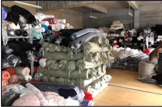
Materials stacked too high, disorganized, unprotected fabric.
