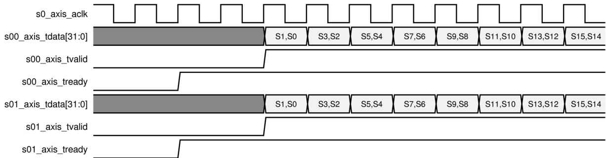
Figure 150: Two RF-DACs with Real Data on Separate Interfaces at 250 MHz
