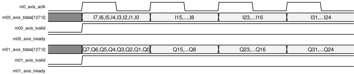
Figure 57: Dual RF-ADC I/Q Input to I/Q Output Timing
